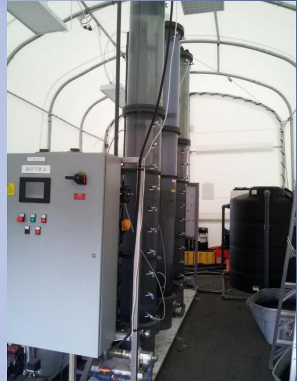
Corollo Engineering Pilot Bioreactor for Nitrate Removal, Delano, California
