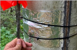
Sap flow sensor in an Aspen tree.
