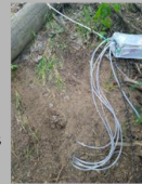
Soil Water Vapor Probes (3 Profiles) ^
