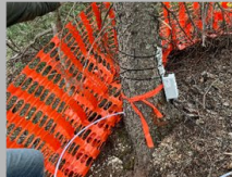
Vapor probe in a spruce tree.
