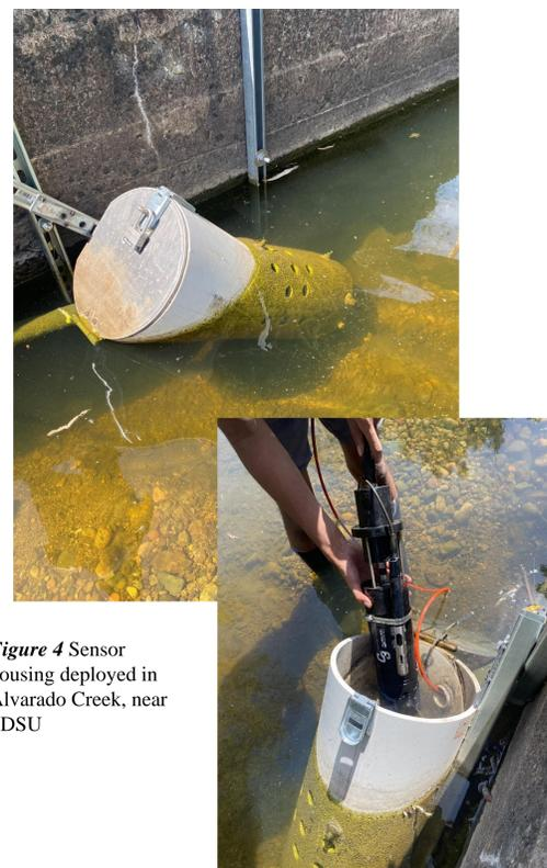
Figure 4 Sensor housing deployed in Alvarado Creek, near SDSU
