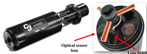
Figure 1 Turner C3 portable fluorometer with three optical sensors
