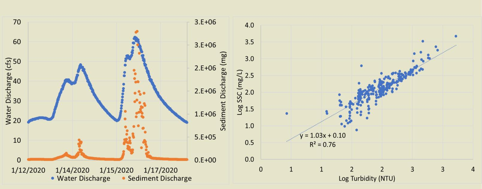
*Figure 5:* Hydrograph and sedigraph for storm 2 which accounted for 57% of the sediment discharged in WY 2020.
