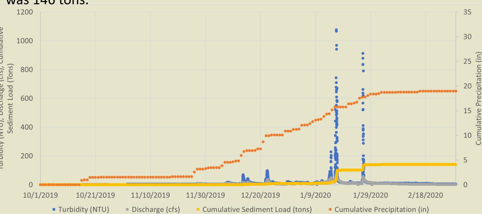
*Figure 3:* Summary of the available site data and analysis for the 2020 water year. The discharge from Salmon Creek is shown in grey, turbidity in blue, cumulative sediment in yellow, and cumulative precipitation in orange.
