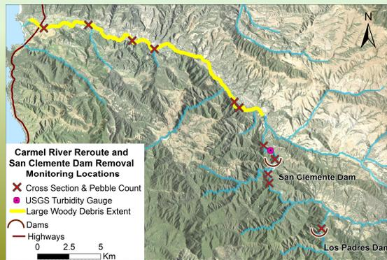
Figure 1. Monitoring locations in relation to the former San Clemente Dam and Los Padres Dam on the Carmel River, Monterey, CA.
