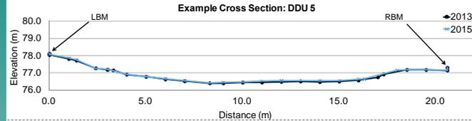
Figure 2. Example cross section (DeDampierre Upper #5) from summer 2013 and 2015, both before dam removal.
