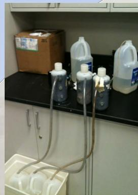
Figure 2: Bioreactor set-up for the project. The columns (from right to left): 1-Woodchips; 2-Woodchips and Sawdust; and 3-Woodchips replicate
