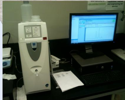
Figure 4: Ion Chromatograph used to analyze the concentration of nitrate in the influent and effluent.
