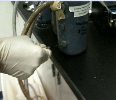
Figure 3: Injection of succinate through the use of rubber ports positioned 1inch apart along the length of the column
