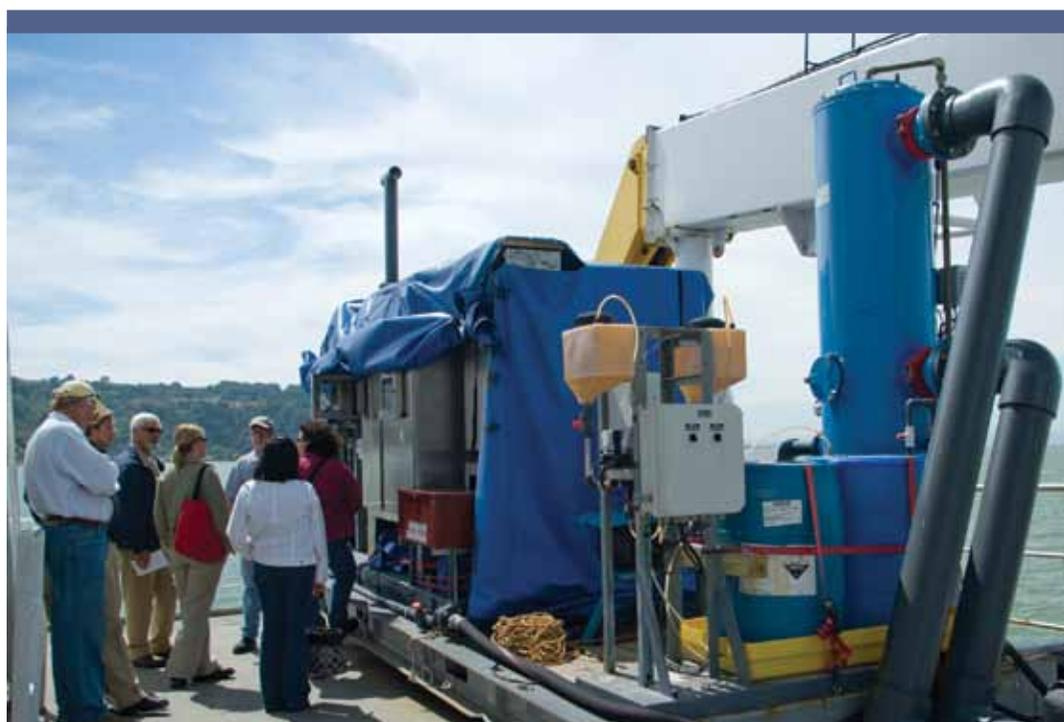
GBF team members and representatives of California State Lands Commission (California's lead ballast water regulation agency) view open-deck installation of the Balpure™ ballast water treatment system on T/S *Golden Bear*. Image courtesy Lynn Takata, CSLC.
